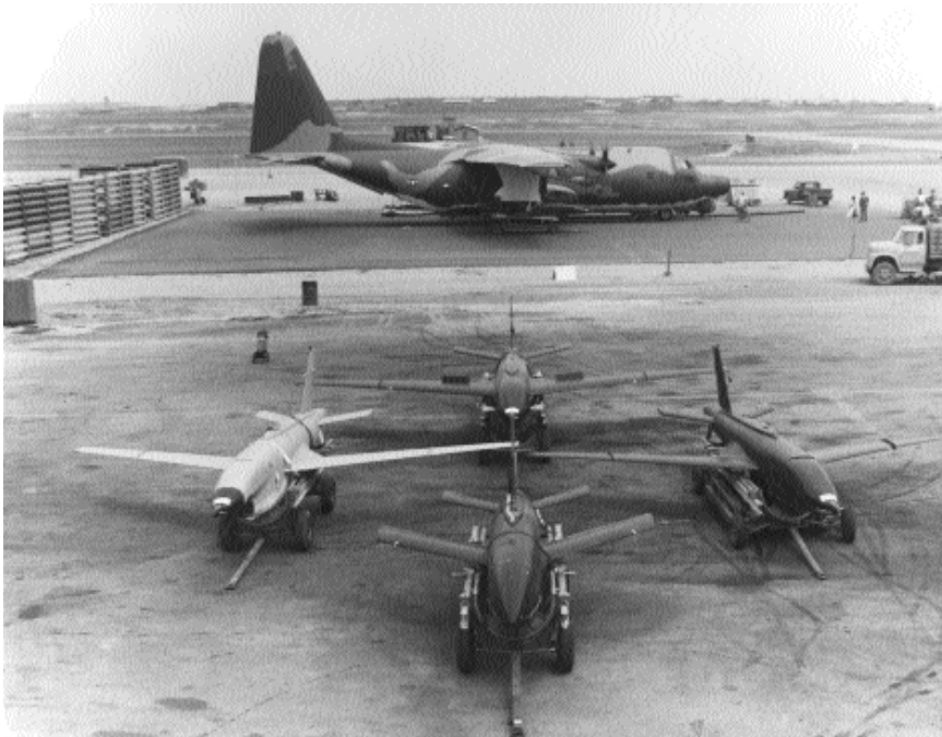
A DC-130 releases a reconnaissance drone (top), and reconnaissance drones with the DC-130 carrier behind them (above).
