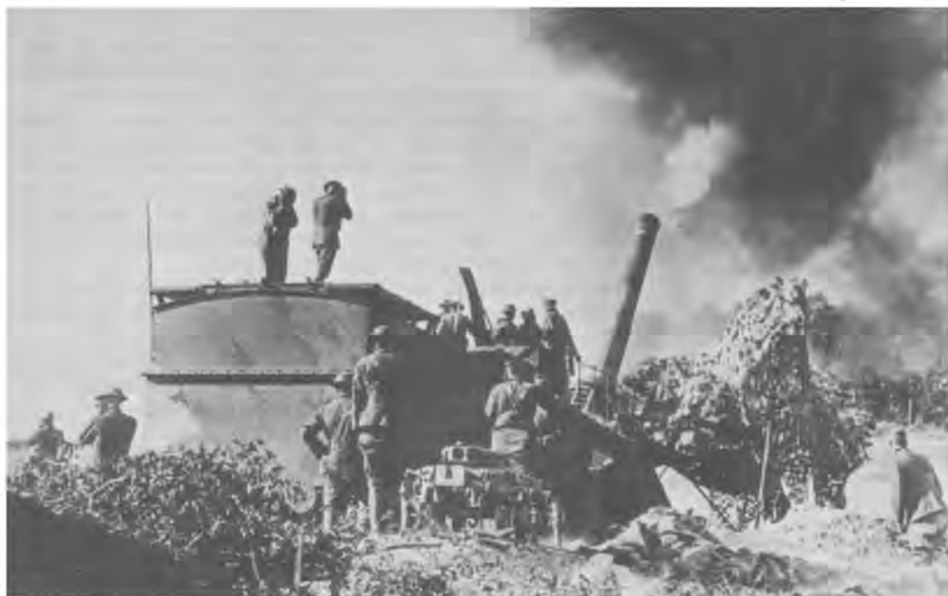
Observers located the disposition of enemy troops for batteries such as this Coastal Artillery at [Nixeville] (Meuse). Shown is a 340-mm railway gun in action.
