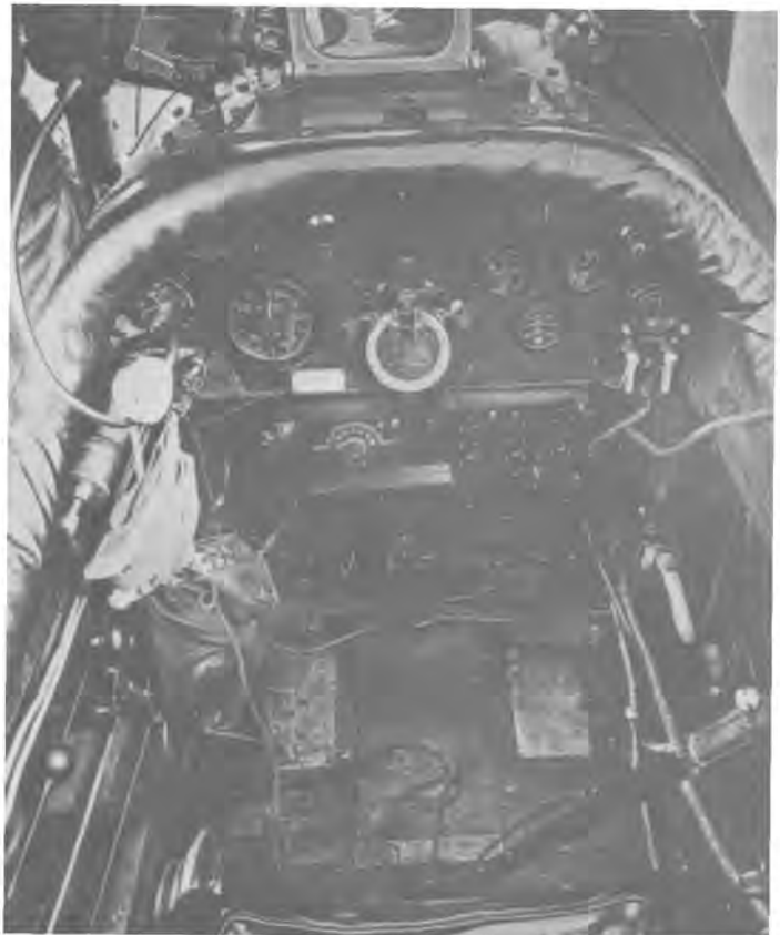
A radio set being installed in a DH-4.
