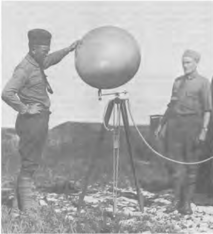
A meteorological balloon to be released for observation in determining speed and direction of wind.
