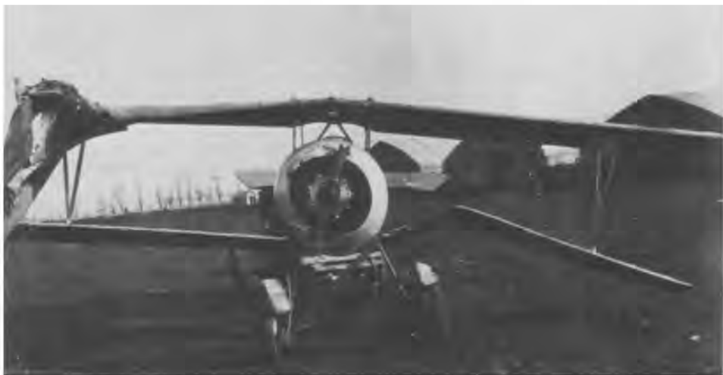
Wrecked airplane, dropped 500 ft. after the motor failed.
