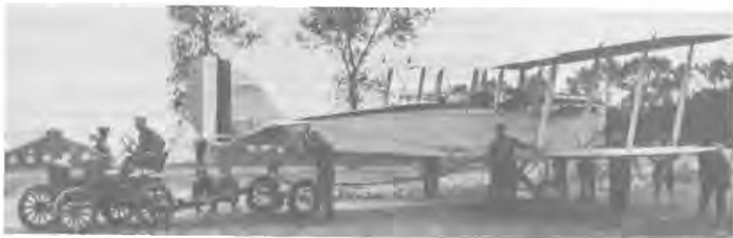
Flight mechanics use a Ford tractor to pull a Liberty plane off the field for maintenance at the Air Service Production Center #2, Romorantin, France.
