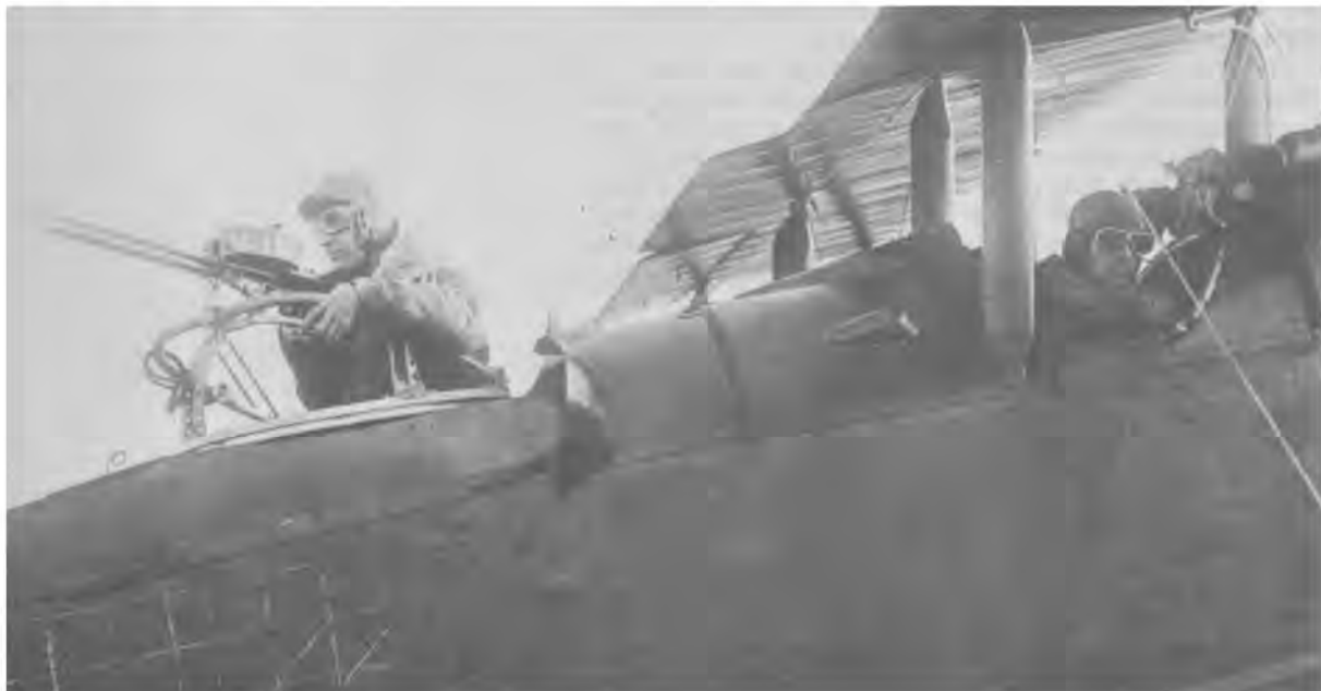
A Lewis gun mounted on a DH-4.
