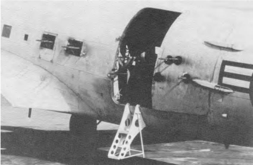
An early AC-47 with ten .30-caliber machineguns mounted for side firing.
