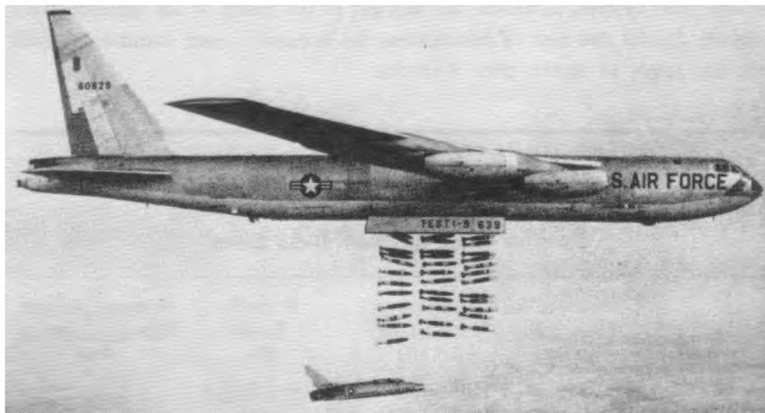
A modified B-52 releases an internal load of 84 bombs in a test over Eglin AFB, Florida, in March 1966 (above). The bomb bay of a B-52 with a load of 84 bombs (right). The bombers can carry 24 more bombs on wing racks.
