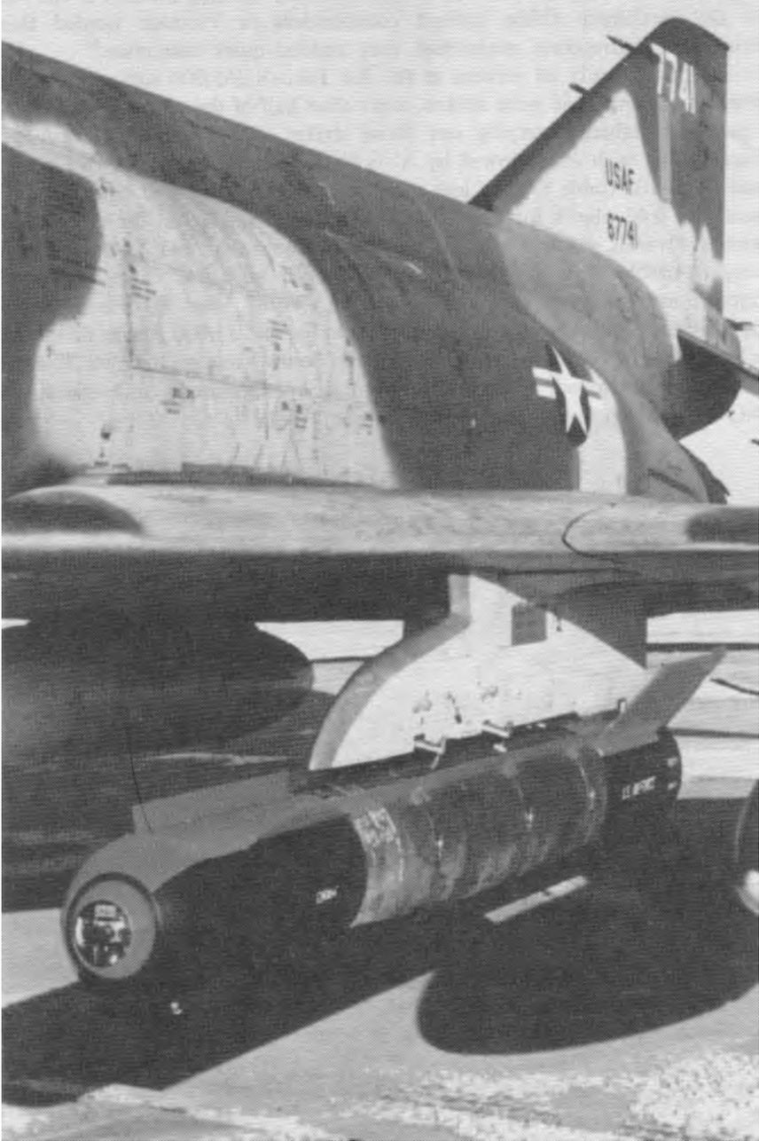
**A highly accurate electro-optical guided bomb on a F-4 Phantom II. Guided bombs were but one class of weapons developed or improved during the war.**
