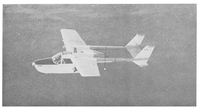
USAF 0-2 "Skymaster" replaced the aging 0-1 as the primary forward air control aircraft
